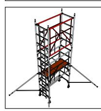
Step 9. Locate next set of AGR panels. Position top hooks of AGR panels on horizontal tubes of the frames before attempting to locate the triggered hooks. Ensure lower hooks are positively locked onto the horizontal rungs and the AGR panels are vertical and parallel to each other
