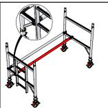
Step 3. Join the second 2 rung frame to the first ensuring brace hook again rests on the first rung of the frame. Fit the second horizontal brace as shown with hook trigger facing downwards. Level around base of tower using spirit level, making adjustments as necessary to adjustable legs until the frames have an inclination no more than 1% from the vertical.
