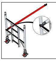
Step 2. Fit a horizontal brace onto the vertical frame tube of the 2 rung frame, resting on the horizontal tube of the first rung of the frame. Ensure the brace trigger faces to the outside of the tower.
